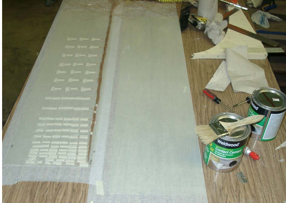
Figure 37. Epoxy board with contact cement. Thermocouple locations can be seen.
