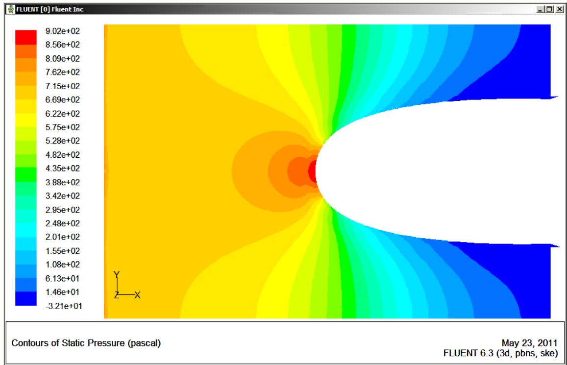
Figure 20. Static pressure contours around the big cylindrical test section from FLUENT.
