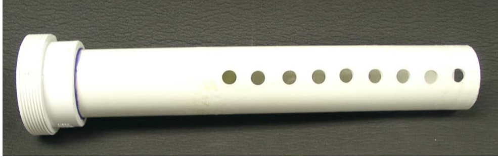
Figure 31. Cool air injection pipe and baffle with quick disconnect PVC coupling.
